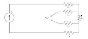
Four Wire RTD: A four wire RTD is the most accurate method to measure an RTD. It is primarily used in laboratories and is seldom seen in an industrial application. A four wire RTD circuit removes the effect of mismatched resistances on the lead wires. A constant current is passed through  $L_1$  and  $L_4$ .  $L_2$  and  $L_3$  measure the voltage drop across the RTD element. The color code for a four wire RTD is usually two red wires and two white wires.
