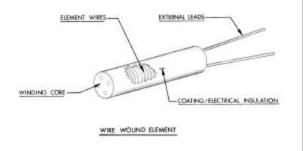
Strain on the element wire will result in an error in the measurement. The winding core must also be selected to match the intended service temperature and environment.
