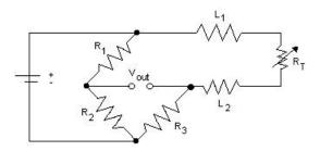
Three Wire RTD: The three wire RTD is the most popular configuration for use in industrial applications. When used correctly, the three wire configuration eliminates the series resistance. This permits an accurate measurement of the sensing element. Two of the leads are connected to one side of the sensing element and the single lead to the other side.
