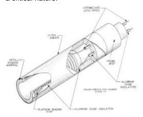
The sensing element is wound on a hollow stainless steel winding core that is insulated with a flame sprayed coating aluminum oxide. A specific stainless steel is chosen for its close match of thermal expansion with the platinum sensing wire. After the usual processing, annealing and coating, the sensing element is enclosed incased with a thin stainless steel sheath. This provides a completely sealed sensing element that can be directly immersed into a process fluid.
